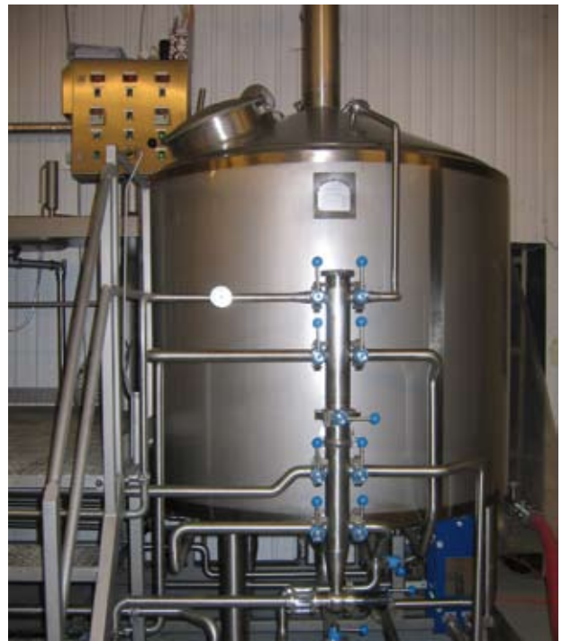
Small matrix of butterfly valves next to the wort kettle/whirlpool.
