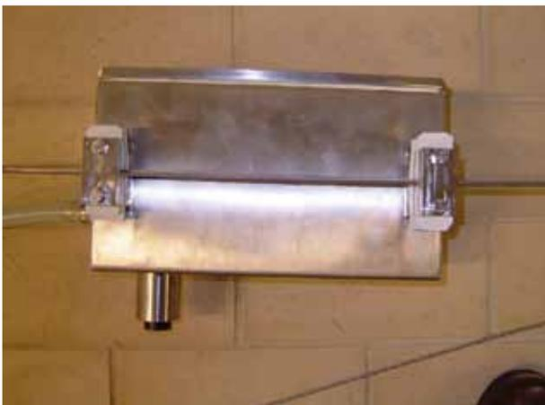
Figure 1. Photograph showing the stainless steel waterproof enclosure surrounding the biomass meter head amplifier and probe. Also shown is the stainless steel cable to which the enclosures were attached.
