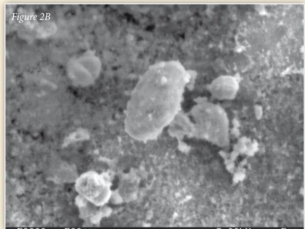
Figure 2. Microbes on stainless steel surface A) in the laboratory and B) on a sample coupon from a one-year process study.
