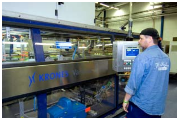
A Variopac TFS 60 with shrink tunnel makes shrinkpacks with or without a tray.
