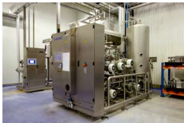
Krones supplied the line complete with the process engineering required: a CIP system and a Contiflow 30/2 beverage preparation system.
