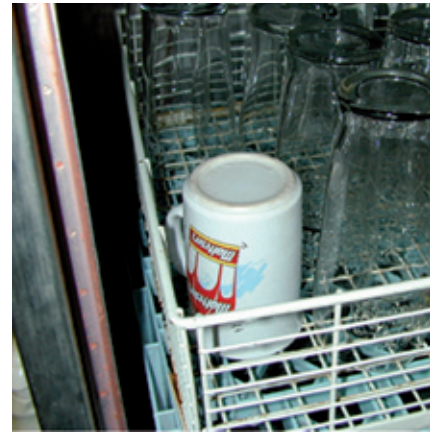
Milk residue from coffee cups contaminates glass washers leading to poor head retention
